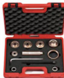
BB TOOL BOX • Multi Functional Tool For Press-Fit BB • Install and remove bearing 6805 (25X37X7) and 6806(30X42X7) • Install and remove press-Fit BB R92/T86 • Install and remove R30(converter for BB30 to BB24) • Weight: 1082g(box included)
