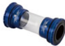
BB-PFS92 • Press Fit External BB set • Shimano System Compatible • 2 sealed Bearings For 86.5mm Road /89.5mm and 92mm MTB • Ceramic Bearing Available • Weight:91g
