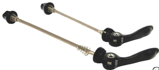
QR-CBF01 Quick release, lever Carbon Axle Cr-Mo * flat * F: M5x112-114mm R: M5x143/148/151mm Weight: 73g
