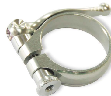
CL-QR03 Quick release for seat Material: CNC 7075 Dia: 40-41mm Weight: 33g
