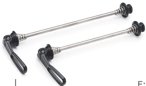
QR-TI01 Quick Release Axle: Titanium Lever: Alloy 7075 Anodized F: M5*112 -114 mm R: M5*143/148/151 mm Weight: 67.4g
